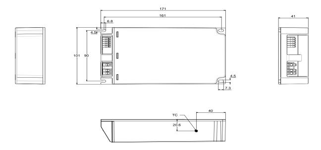
Notes: EQUI pin connects to ground wire and metal housing of luminaries for Class I applications, and to metal housing for Class II applications.
