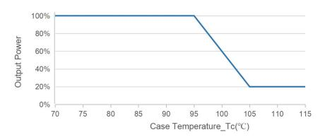
Notes: Customers can set the start derating temperature and end derating temperature. This curve is the default factory protection curve, When the temperature rises to the normal operating temperature, the drive will resume output.
