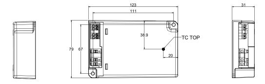
Notes: EQUI pin connects to ground wire and metal housing of luminaries for Class I applications, and to metal housing for Class II applications.
